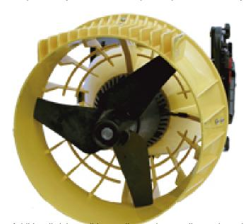
Additionally it is possible to easily vary the propellers angle or pitch, which allows for even more fine-tuning of the scooters speed to the individual divers needs.
